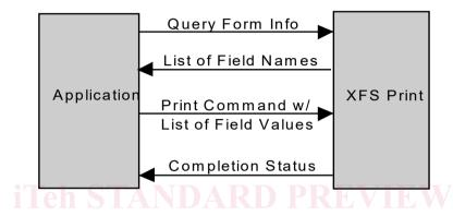
The XFS implementation recognizes that the form object must be supported by job-specific data to fully address printing requirements. As an example, a form defining a passbook print line will need to have its origin defined externally in order to be reused for different passbook lines. These job specific parameters are supplied on the call to the **WFSExecute**: WFS CMD PTR PRINT FORM command.
