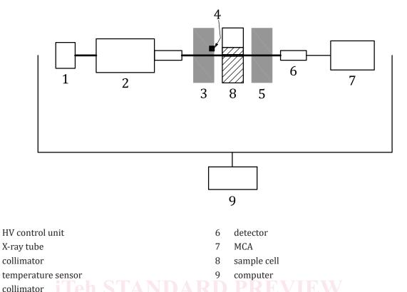
Figure 1 — Schematic of the instrument components
