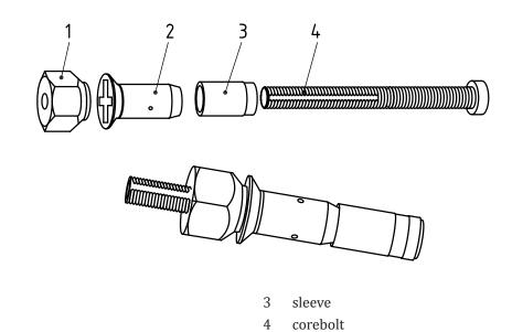
Figure 1 — Blind fastener, threaded type
