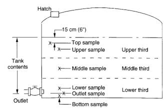
Note 1—The location shown for the outlet sample applies only to tanks with side outlets. It does not apply when the outlet comes from the floor of the tank or turns down into a sump. Bottom sample location must be specified.
