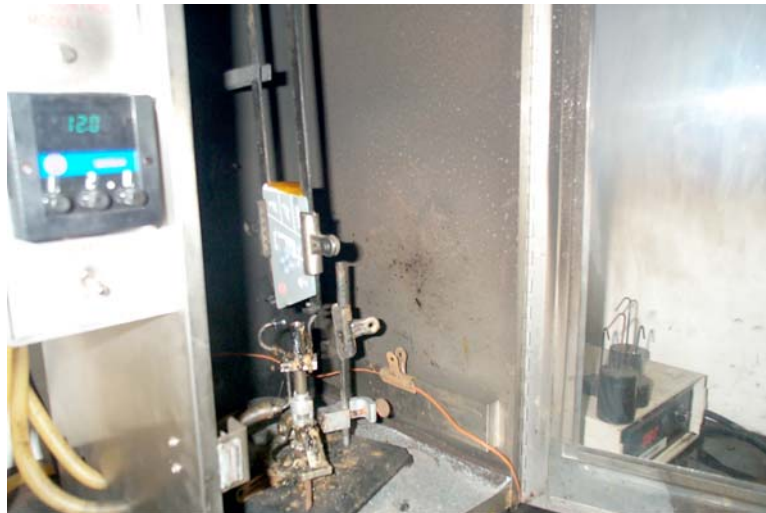
FIG. 1 Typical FPA Test Booth
