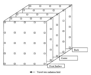
Note 1—In this drawing the small squares represent dosimeter positions. The "Front" is defined as the initial and in some cases only surface to directly face the radiation source during processing. The number of dosimeters and the number of planes (surfaces) to be mapped will depend on several factors, including but not limited to, the radiation type (electrons versus photons), single- versus double-sided irradiation, and resolution of absorbed dose required.
