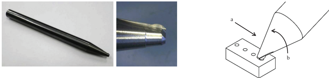
a) View of cutting tool (left) and enlarged view of cutting tip part (right)
