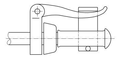
Figure 3 — Method of fitting the gauge to the brake-lever and handlebar
