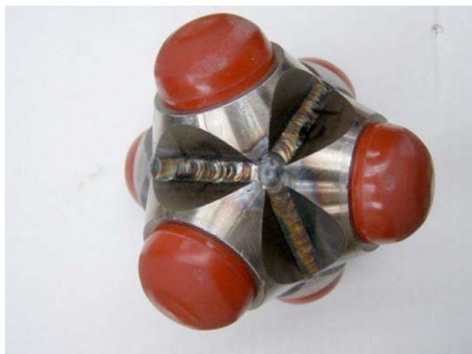
FIG. 3 8.4 lb Commercial Hexapod Tumbler
