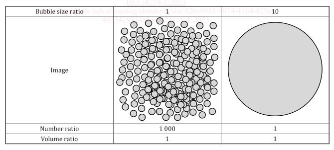
Figure 1 shows the two types of size distribution graphs of bimodal which are equivalent, but the impressions are very different as dimensions such as number and volume are different.
