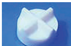
Figure 1 — Cowie double cross-head stir bar (typical dimensions: 20 < d < 25\ \text{mm} , 12 < h < 18\ \text{mm} )
