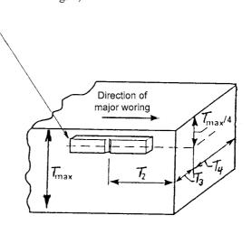
Note 1—For material with thickness *T* greater than 2 in. [50 mm],  $T_2=T_3=T_4 \ge T_{\text{max}}$ where:
