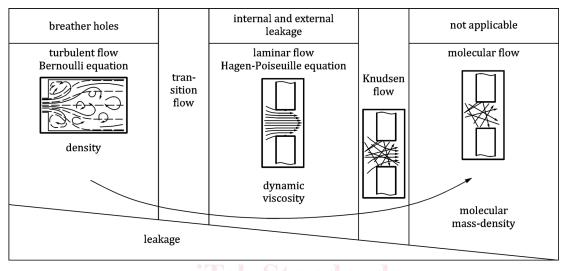
To avoid too much damping on the regulator, breather holes need to have a certain minimum size. That is, the flow can turn from laminar to turbulent, because breather hole sizes are bigger than internal/external leakage hole sizes.
