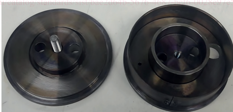
Figure 1 — Typical mould assembly - Left: bottom plate - Right: Inner and outer rings placed on the top plate (step D of 4.3.1 )
