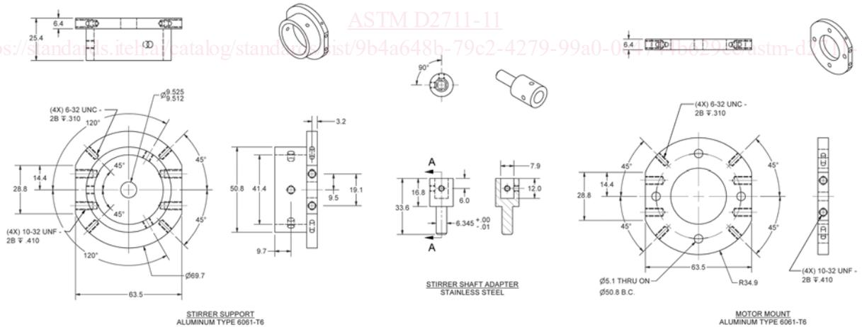
FIG. 3 Detailed Construction of Stirrer, Part 2
