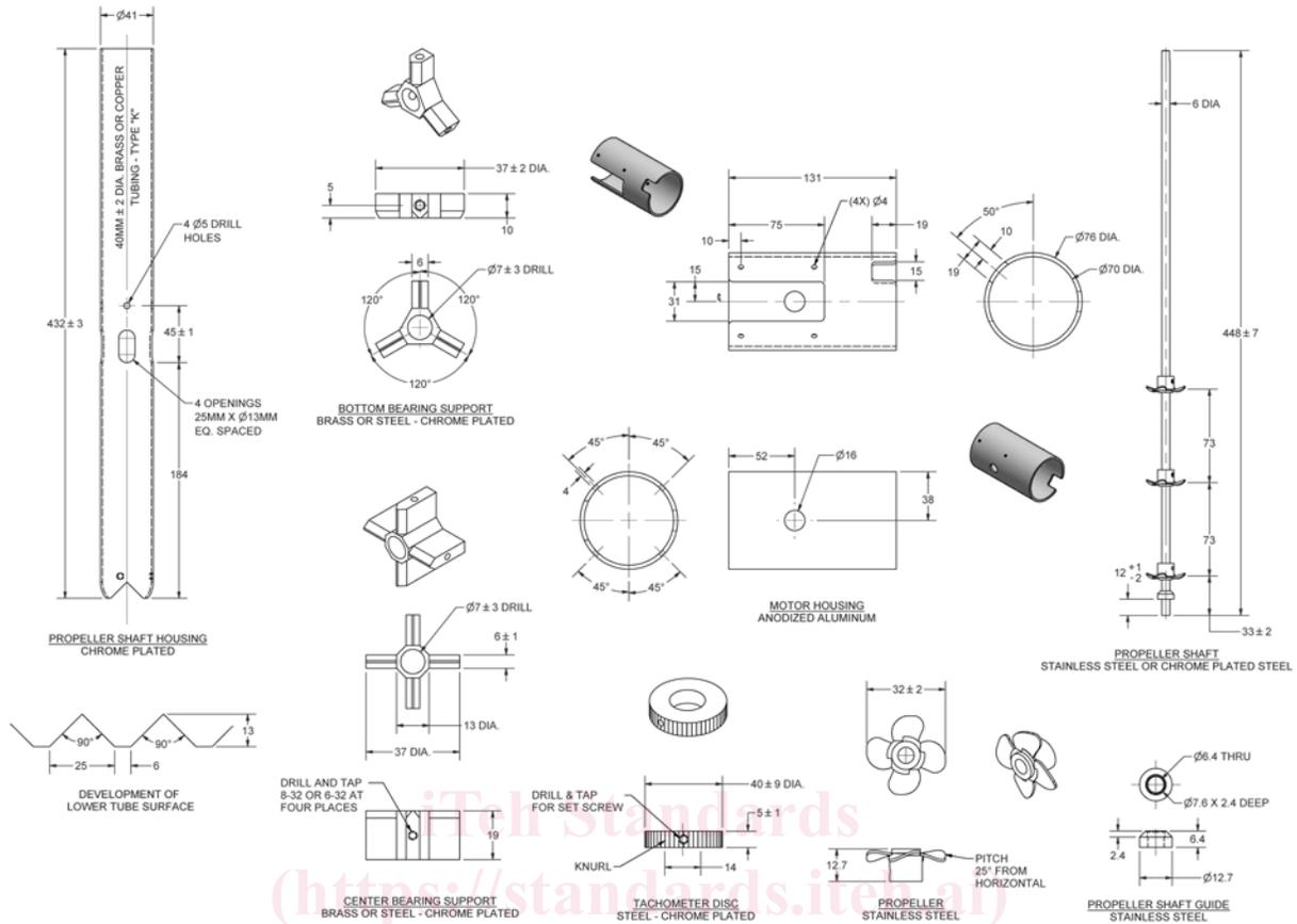
FIG. 2 Detailed Construction of Stirrer, Part 1
