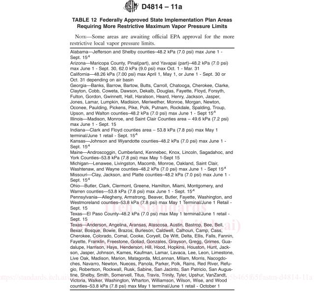
$^{A}\,A$  1.0 psi higher vapor pressure is allowed for gasoline-ethanol blends containing 9 to 10 volume % ethanol.
