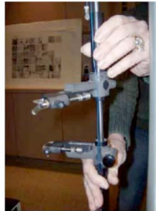
b. Photograph of Cable "Roller Style" Extensometer
