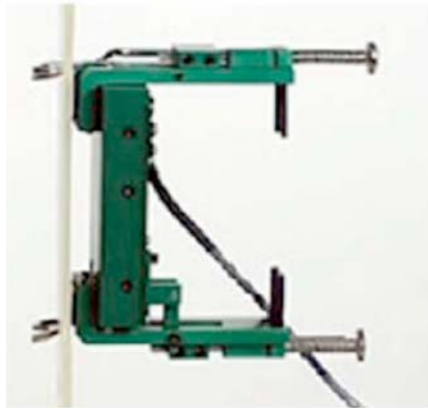
a. Photograph of Clip-On Extensometer
