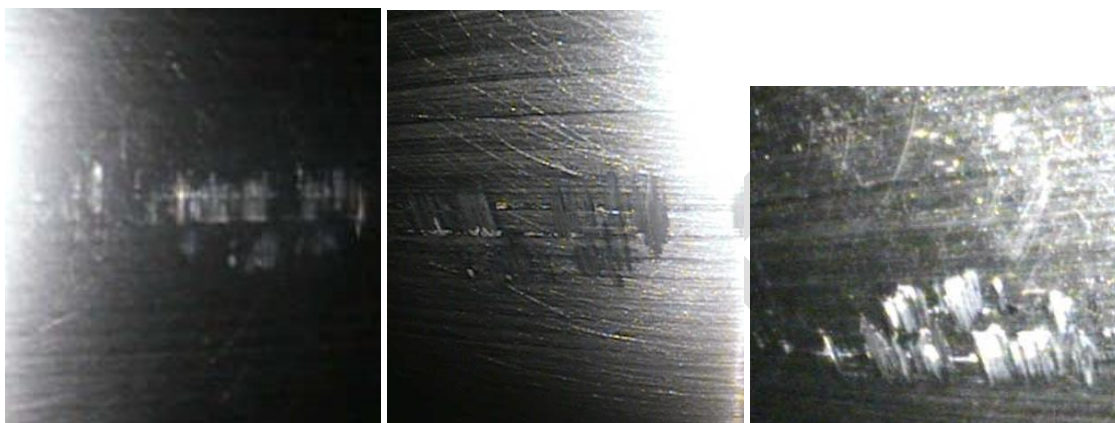
Figure 7 – Three body abrasive wear
