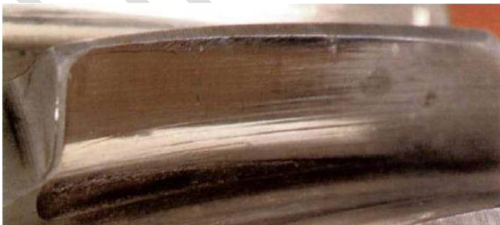
Figure 4 – Severe polishing on a misaligned gear
