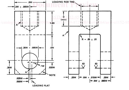
A – SURFACES MUST BE FLAT, IN-LINE & PERPENDICULAR, AS APPLICABLE TO WITHIN 0.002 IN T.I.R. (.05 mm)
