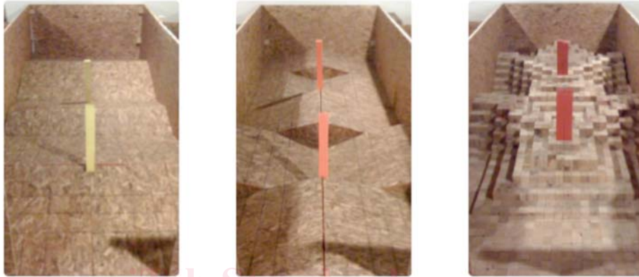
FIG. 1 Mobility: Confined Area Terrains: Crossing Pitch/Roll Ramps Apparatuses
