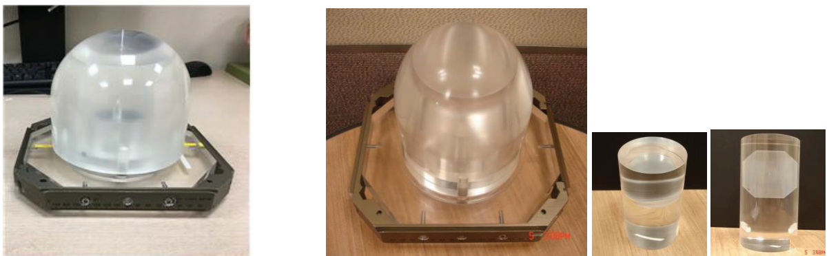
a) Photographs of the ionization chamber insert of the Gamma Knife® polystyrene phantom
