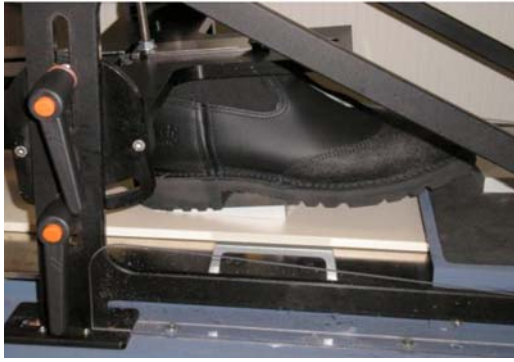
FIG. 1 Example of Footwear Mounted Using 7° Wedge to Set Proper Contact Angle
