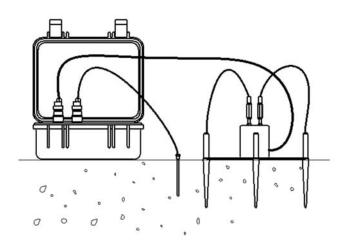
Note—The wires crossing in the diagram are not touching each other during use to prevent parasitic capacitance.
