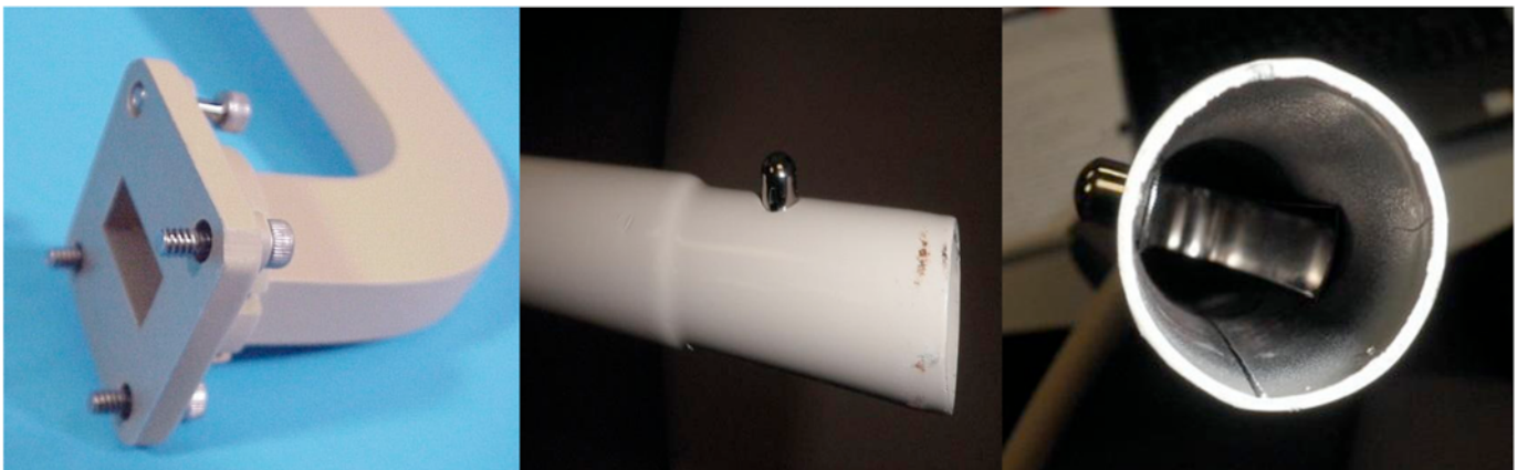
Bolt is free floating, can retract but not completely removable
