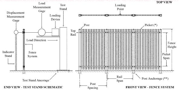
\* Note I - Any picket point style is acceptable on tested system; pickets may extend through the rails (as shown) or may terminate at
