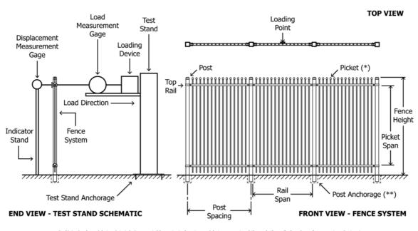
\* Note 1 - Any picket point style is acceptable on tested system; pickets may extend through the rails (as shown) or may terminate at the rails. Range of qualification is based on maximum picket span.
