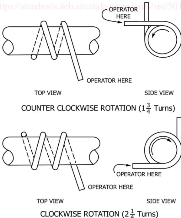
FIG. 1 Number of Rope Turns on Cathead
