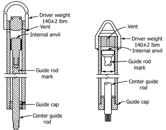
FIG. 2 Internal Anvil Safety Hammers—Typical Designs
