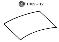
chip—area along an edge or corner where the material has broken off.
