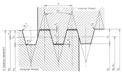
1) It is recommended to provide for a rounding or a chamfer equal to  $0.5 a_c$ or less at the major diameter of the external threads. For rolled screw threads with pitch 2 to 12, it is recommended to provide for a rounding or a chamfer equal to  $0.6 a_c$  or less at the major diameter of the external threads.
