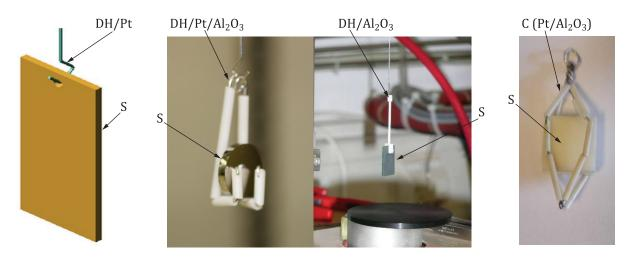
a) Using a hole drilled b) Using a hole drilled c) Using a hole drilled d) Using a platinum/ in the specimen in the sample and a in the sample and an and a Pt wire to hold platinum/alumina sam- alumina sample holder the specimen ple holder
