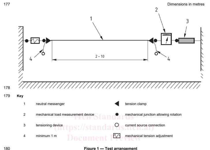
Figure 1 — Test arrangement
