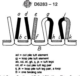
FIG. 1 Cross-Section of Tufted Pile Yarn Floor Covering
