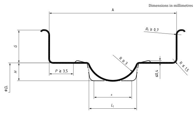
The tyre bead seat must be parallel to the rotational axis of the wheel.
