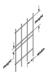
Note 1—Model A panels normally have horizontal reinforcing folds (or beams) to increase horizontal rigidity. Number of folds (beams) increase with the height of the panel. Generally two folds for panels shorter than 5 ft [1525 mm], three folds if shorter than 6 ft 6 in. [1980 mm] and four folds for taller panels up to 8 ft [2430 mm].
