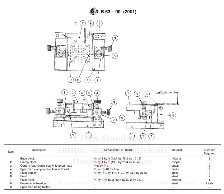
Note 1—Contact surfaces must be clean and free of visible oxide. FIG. 1 Specimen Holder for Nonductile Materials
