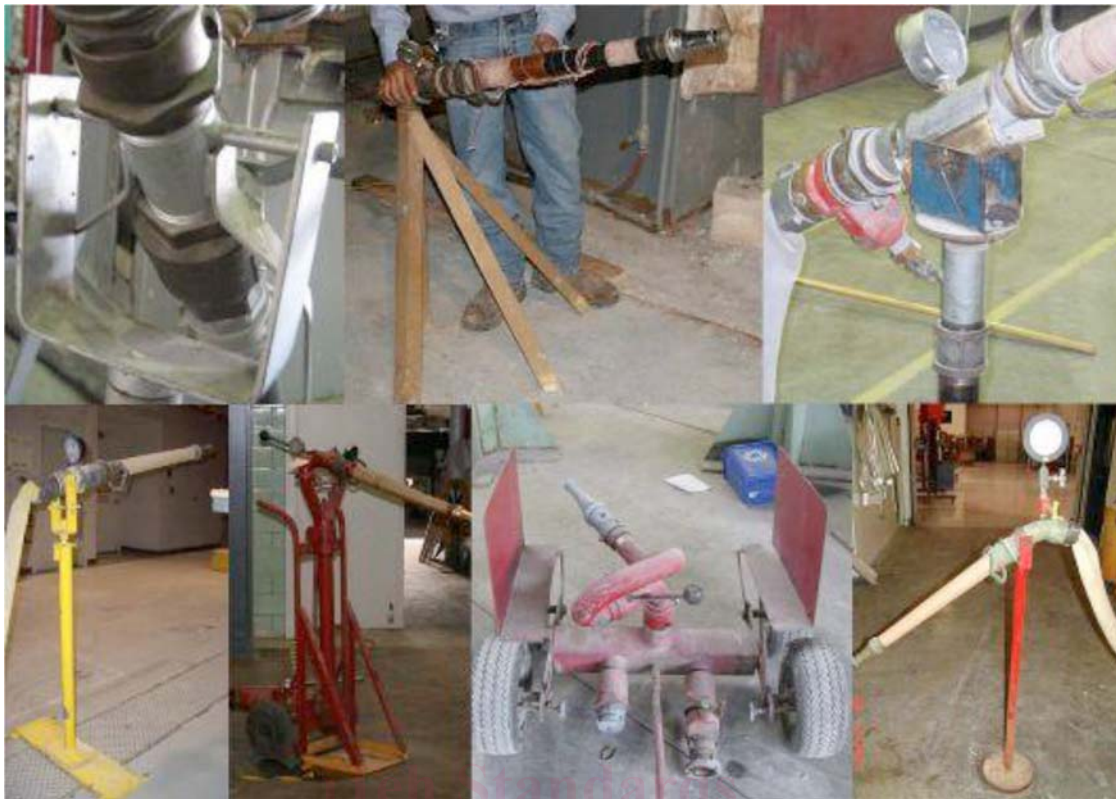
FIG. 2 Typical Hose Mounting Methods
