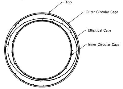
Note 1-The total reinforcement area of the inner circular cage and the elliptical cage shall not be less than that specified for the inner cage in Tables 1-5
