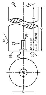
Note 1—Opposite ends of reference block shall be flat and parallel within 0.001 in. [0.025 mm].
