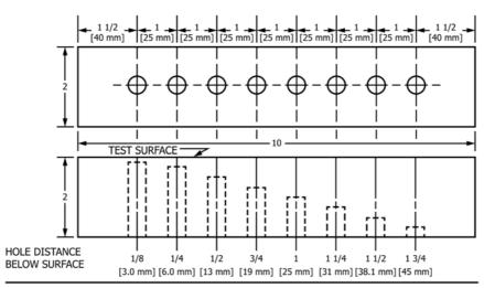
Note 1-Entrant surface shall be 250 µin. [6.3 µm] or finer.
