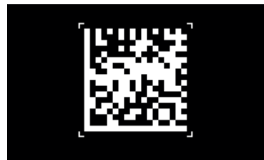
b) Data Matrix, light on dark (reflectance reversal)
