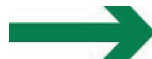
Figure 1 — Arrow indicating the direction of movement of people for displaying the primary escape route
