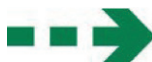
Figure 2 — Arrow indicating the direction of movement of people for displaying the secondary escape route
