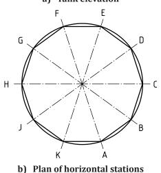
NOTE The horizontal stations are designated A to K in the plan view (see also 6.4.2). Of these, only E and F are shown in the elevation.
