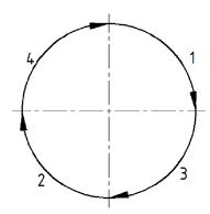
NOTE 1 Ensure that alternate sections of the circumference are welded in sequence as shown to avoid heat deformation. Weld the  $90^{0}$  shown as "1", skip  $90^{0}$ , then weld section "2". Skip  $180^{0}$  and weld section "3". Skip  $90^{0}$  and weld section "4", the last section.
