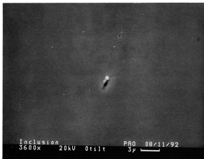
FIG. 2 Example of Pit Defect (3600 × magnification)
