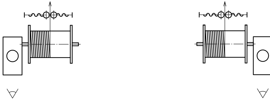
a) Left-hand winch of horizontal spooling rope b) Right-hand winch of horizontal spooling rope
