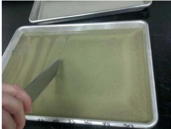
FIG. 1 Full-Depth Cut in Test Specimen
