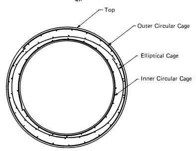
Note 1—The total reinforcement area of the inner circular cage and the elliptical cage shall not be less than that specified for the inner cage in Tables -5.
