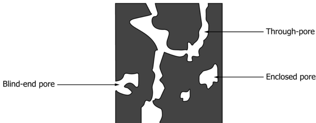
FIG. 5 Schematic Representation of Different Pore Types that Can Exist within a Tissue Scaffold
