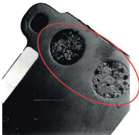
Figure 6 — Poor consolidated spigot holes
