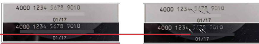
Figure 3 — 50 cycles before (left) and at (right) stopping point for resin-based text
